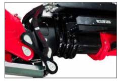
LINKAGE on crane articulation, maintaining a constant lifting moment and better crane performances in terms of both dynamic lifting and static capacity.
